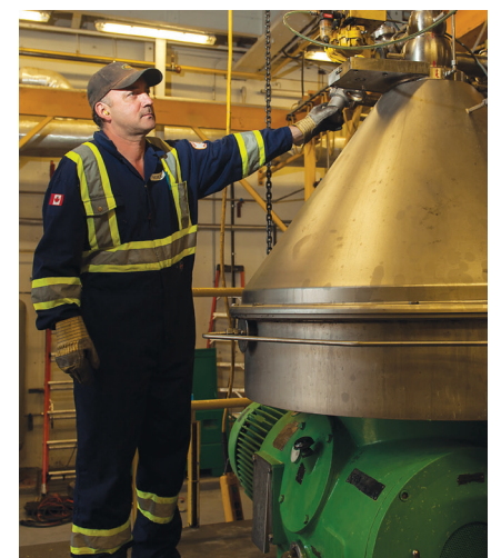
Located at the Port of Vancouver, these centrifuges are used to extract recycled oils and fats as well as manufacture feedstocks for biofuels.
